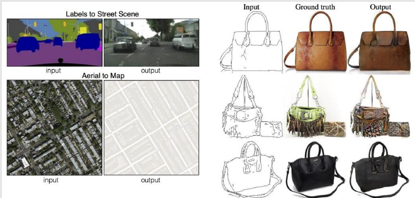
Figure 7: Isola et al. (2016) created a concept they called image to image translation, encompassing many kinds of transformations of an image: converting a satellite photo into a map, converting a sketch into a photorealistic image, etc. Because many of these conversion processes have multiple correct outputs for each input, it is necessary to use generative modeling to train the model correctly. In particular, Isola et al. (2016) use a GAN. Image to image translation provides many examples of how a creative algorithm designer can find several unanticipated uses for generative models. In the future, presumably many more such creative uses will be found.
