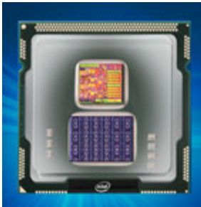
Loihi 2017 (Intel) On-chip learning Fully digital 131,072 neurons, 130M synapses
