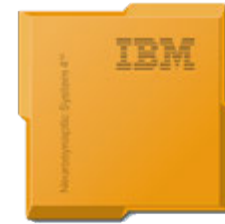
TrueNorth 2014 (IBM) Fully digital 1M neurons, 256M synapses 25 pJ (energy/connection)
