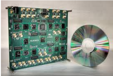
Neurogrid 2009 (Stanford) Analog, sub-threshold 1M neurons, 4B synapses 100 pJ (energy/connection)
