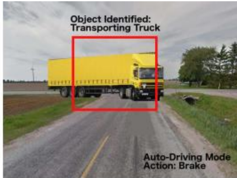
(a) Fault-free execution: A truck is identified by the DNN and brakes are applied
