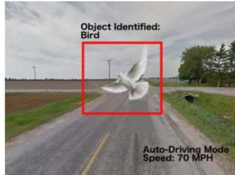
(b) SDC: Truck is incorrectly identified as bird and brakes may be not applied
